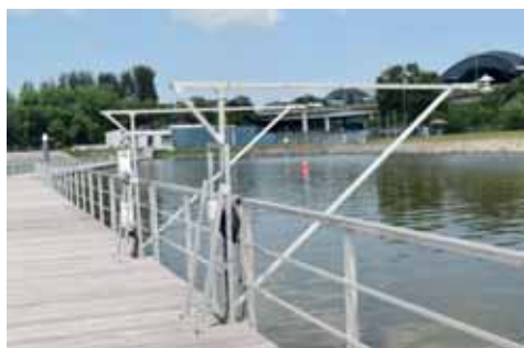
Figure 13. Albedo measurements on water
