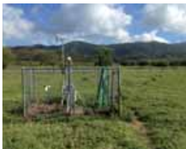
Figure 7. Example of a solar monitoring system with pyranometers and associated weather equipment.
