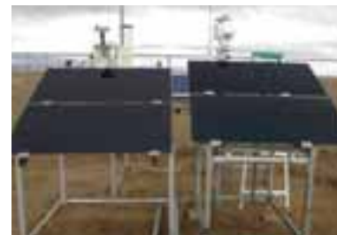
Figure 9. Examples of a reference cell and reference modules in the field.
