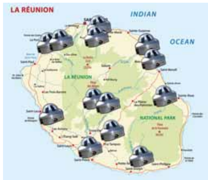
SPN1 network on Reunion Isle in the Indian Ocean – used to study solar resource variability, and the implications of a high proportion of renewable energy for managing the electricity grid.
